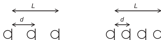
Figure 8. Illustration of the reduction in microphone distance d with adding more microphones, when total array length L is fixed.
