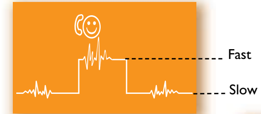
DFC uses two reaction modes. It reacts slowly to small, slow alterations such as the ear mould or custom instrument changing position. This ensures good everyday sound quality. For larger, sudden changes such as answering or terminating a phone call DFC switches to fast mode and reacts in a matter of milliseconds.
