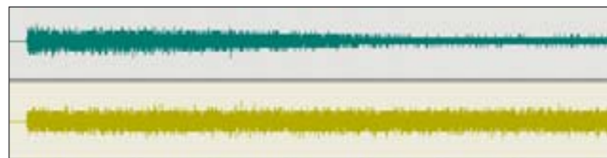
Amigo’s output from a white noise input with Noise Management on (Top) and off. The attack time from the detection of the unmodulated noise until reaching a steady state is about 5.5s.
